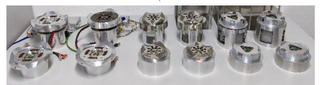
Fig. 6 In the context of the Project PERIOD with Benchmark tested SIs mounted on adapters from left to right: iSSI<sup>®</sup> active and passive with optional formfits [5], HOTDOCK active and passive [4] and SIROM active and passive [6]. The active type SI are in the back row and the passive SIs are in the front row.
