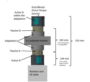
Fig. 8 Fixed distances of the test setup.
