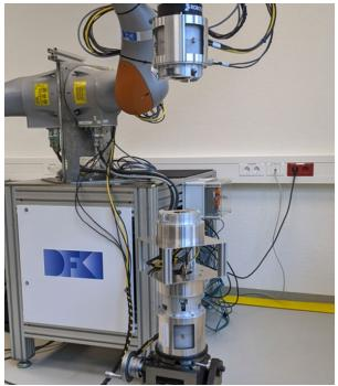
Fig. 9 Test setup with fixed bottom payload module.
