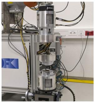
Fig. 10 Test setup with fixed payload module on the end-effector of the Kuka arm
