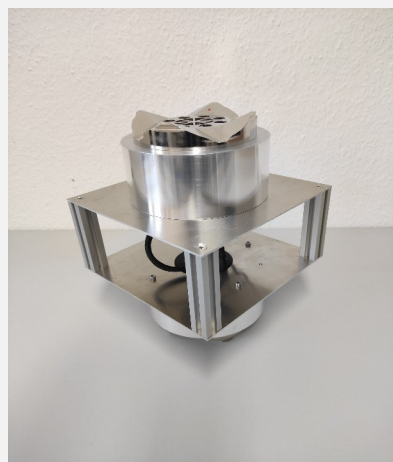
Passive HOTDOCK on 4U payload mockup
