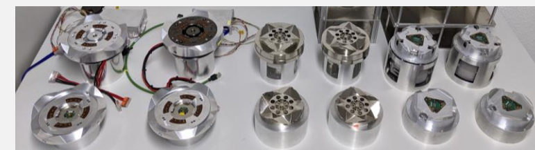
Tested SIs mounted on adapters from left to right: iSSI® active & passive with optional formfits, HOTDOCK active & passive and SIROM active & passive.
